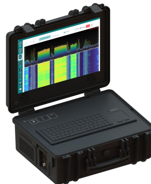
MGI with down converter and A 5.1 decipher inside
